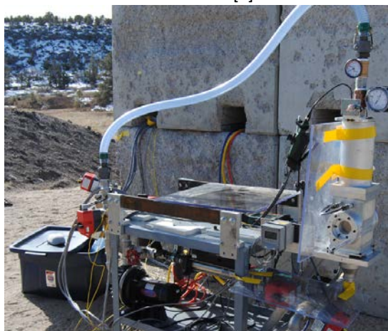
FIGURE 1. Rubidium metal target failure test bed designed to simulate the target environment during failure. The mockup target station is on the right.
