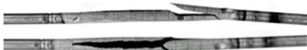
Fig. 1: Post-test appearance of the rodlet VA-1, which was tested in a RIA simulation test in the NSRR reactor in Japan [1].
