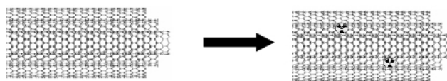
Fig. 2: 7 Be implantation in MWCNTs via proton irradiation of 7 Li and recoil labeling.
