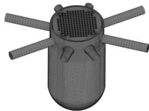
Fig. 3: Outline of the ROCOM ANSYS-CFX calculation grid.
