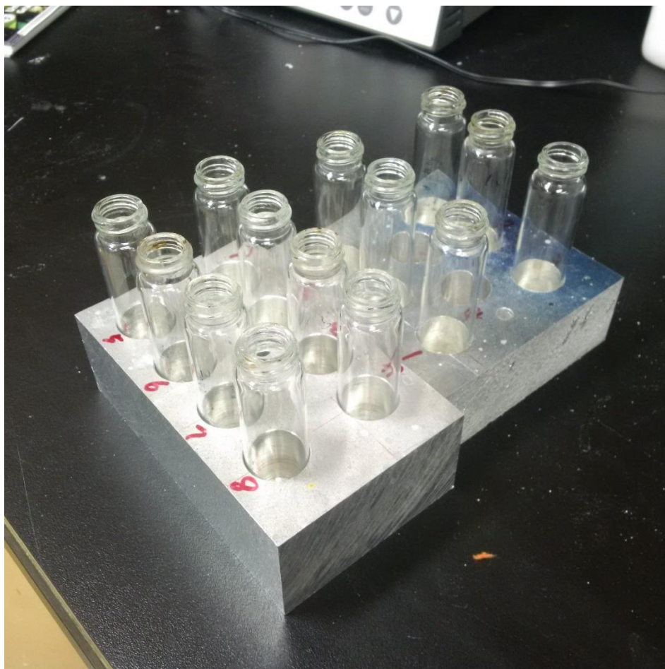
Figure 3.2 Customized block heater for fatty acid extraction
