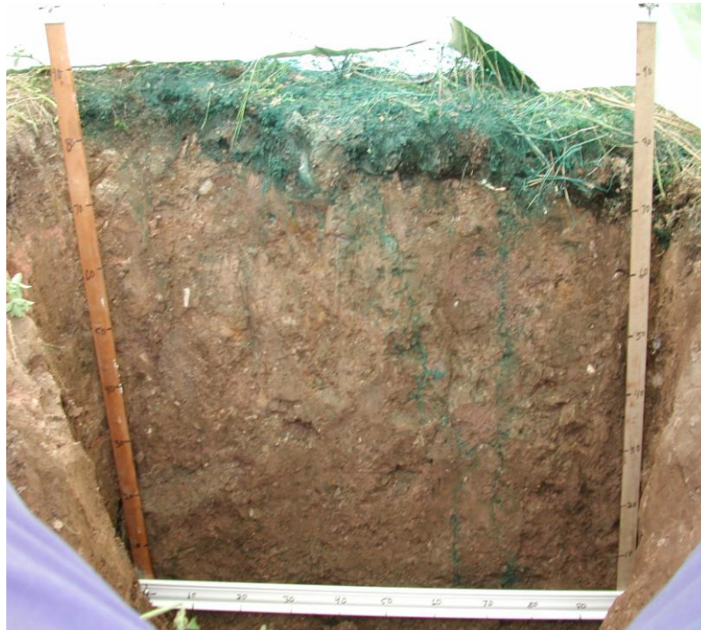
Figure 3.7 Vertical flow patterns of Brilliant Blue dye, and the matching one-dimensional profile of dye coverage, one day after soil plots were irrigated with a total application of 0.04 m dye solution. Profile shown is representative of the middle slope position of the 1-m soil cover.
