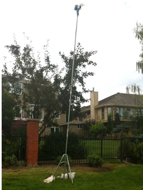
Figure 3-22. Camera set up at an oblique angle overlooking the stormwater pond with the drogues in the flow.
