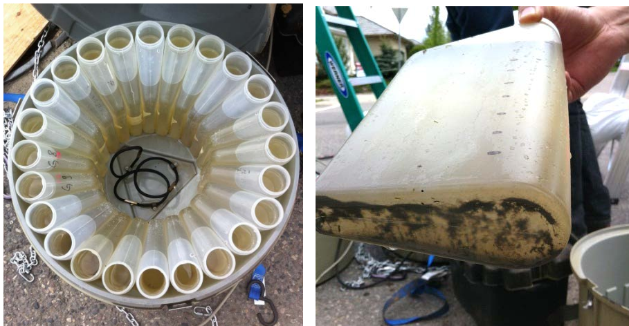
Figure 3-10. (Left) Retrieval of ISCO 6700 samplers for data logging, sample bottle exchange and battery exchange (center), and return to the manhole (right).
