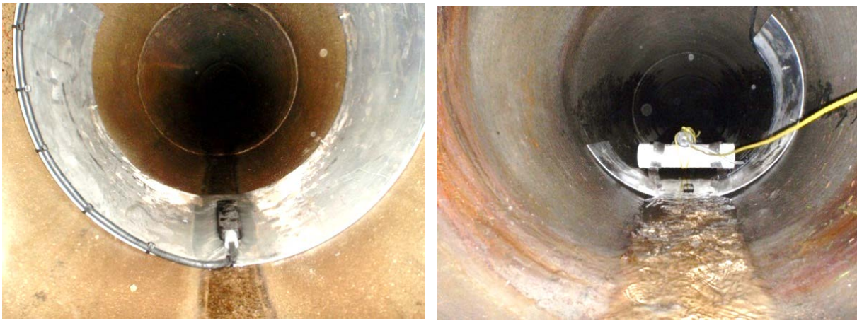
Figure 3-6. ISCO 750 area-velocity modules installed upstream of the intake strainer initially used for the project.
