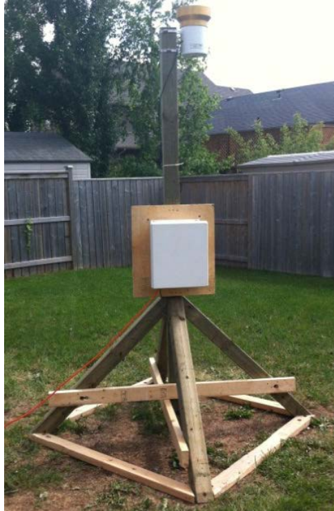
Figure 3-2. Tipping bucket rain gauge mounted to a stand along with the data logger protected in an enclosed box.
