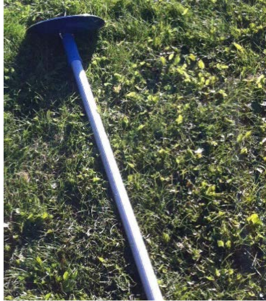
Figure 3-17. Telescopic pole with metal foot used to take depth to sediment surface measurements.
