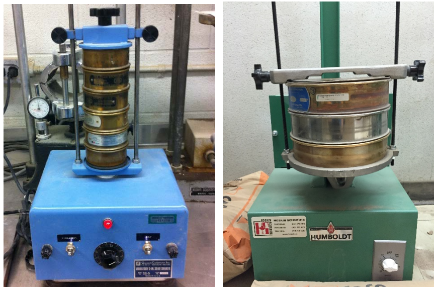
Figure 3-12. Gilson Vibratory Sieve Shaker (left) and Hoskin Scientific mechanical sieve shaker (right) used for particle size distribution testing of solids.
