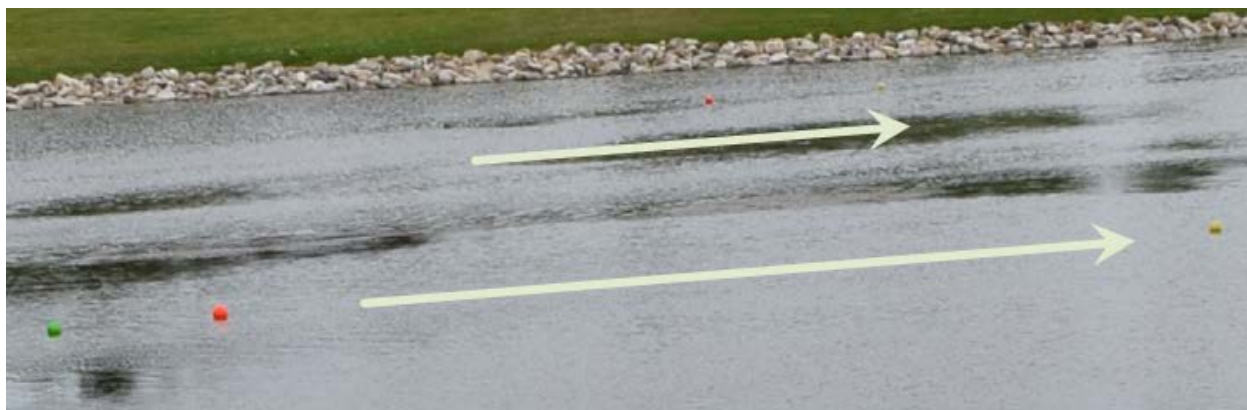
Figure 4-26. Drogue tracking showing the leading drogue with the shallowest fin, with drogues with deeper fins lagging in order of depth.
