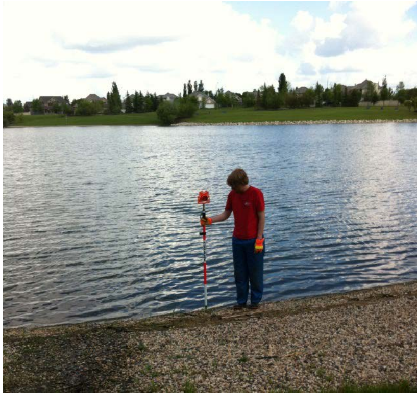
Figure 3-19. Surveying the water elevation of the pond as part of the sediment depth measurement procedure.
