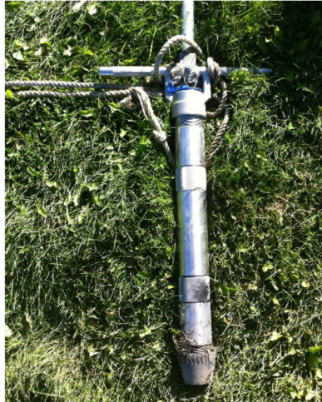
Figure 3-16. Wildco hand corer with extension pole attached, used to take core samples of pond sediment.
