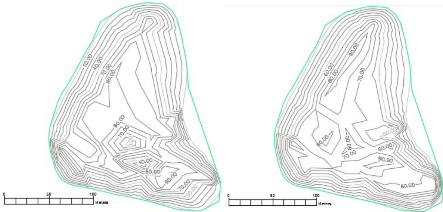
Figure 4-17. Percentage of sand by mass throughout the pond, from June (left) and August (right) measurements (10% contour intervals)
