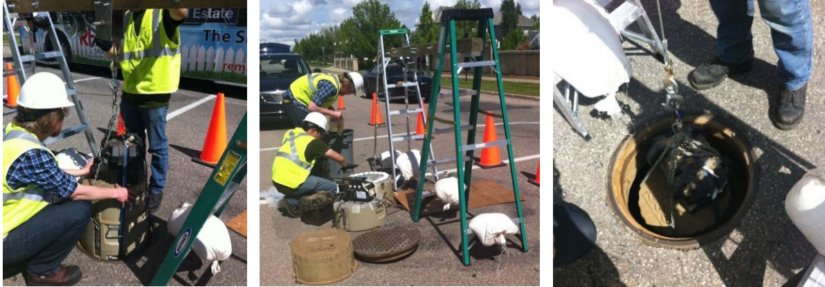
Figure 3-10. (Left) Retrieval of ISCO 6700 samplers for data logging, sample bottle exchange and battery exchange (center), and return to the manhole (right).
