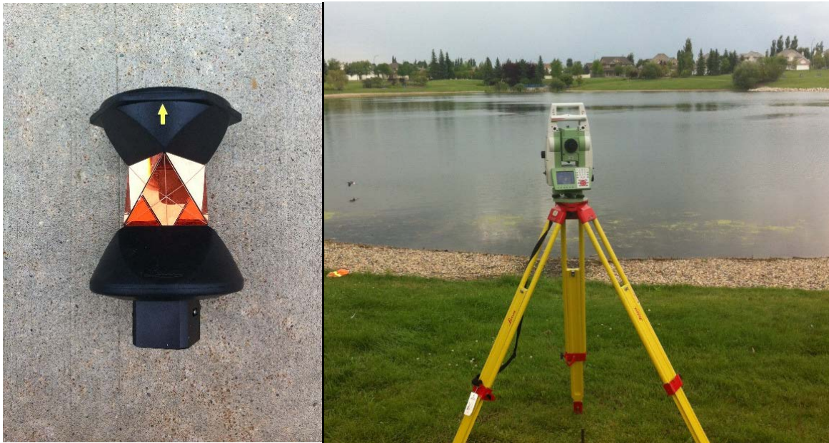
Figure 3-21. Three-dimensional prism (left) and Leica robotic total station (right) used to track the prism-attached drogue.
