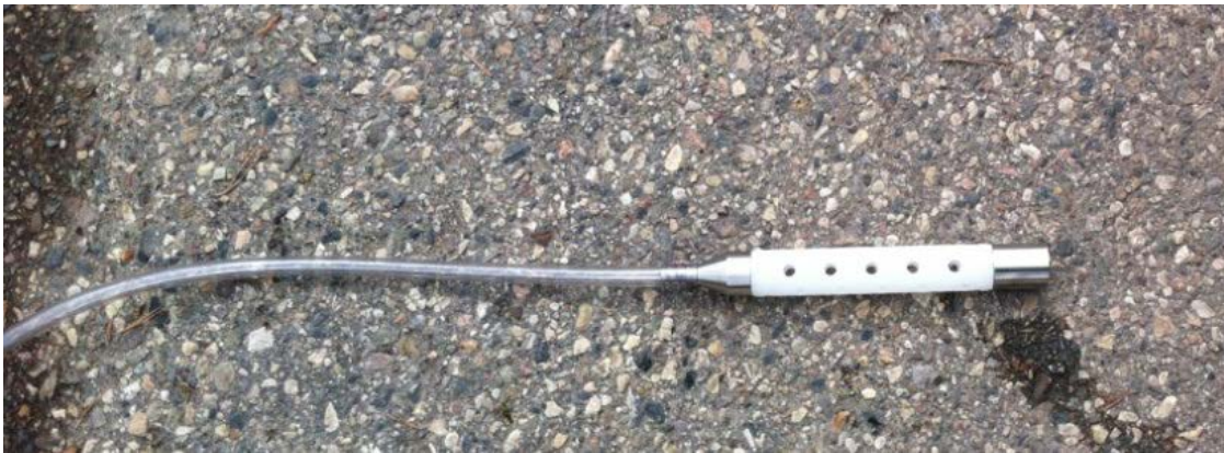
Figure 3-4. Manufacturer's intake strainer for stormwater to enter the ISCO sampler pumping system.
