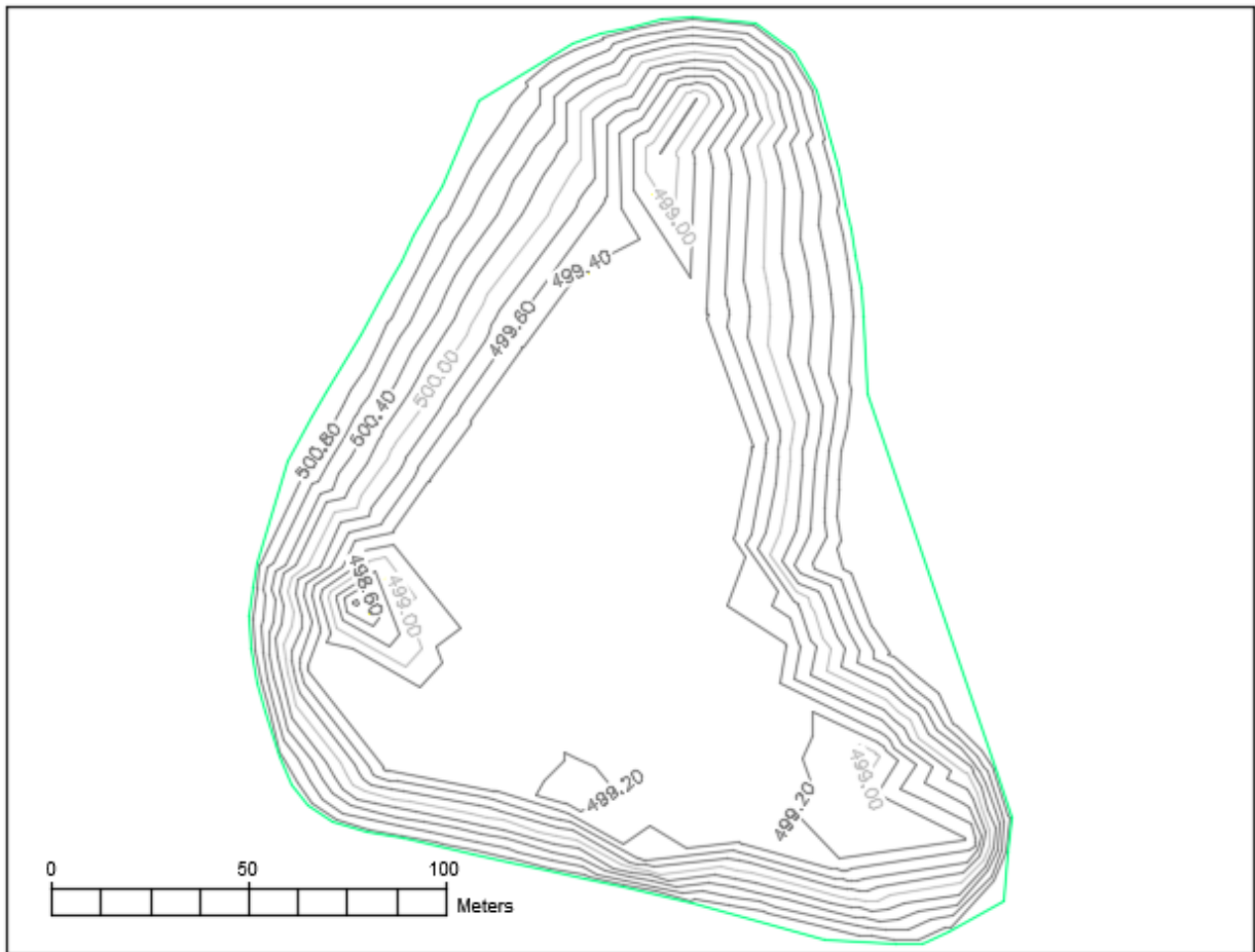
Figure 4-15. Measured in August existing pond bottom elevations with a 20 cm contour interval, where the design pond bottom elevation was 499.0 m.
