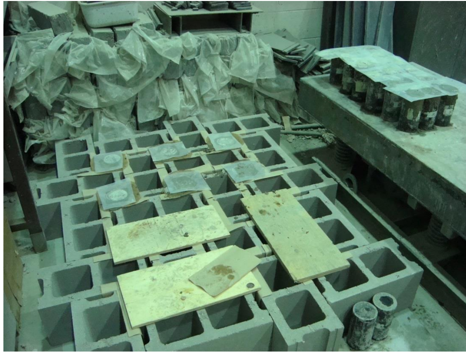
Figure 3.12. Preparation of grout companion specimens
