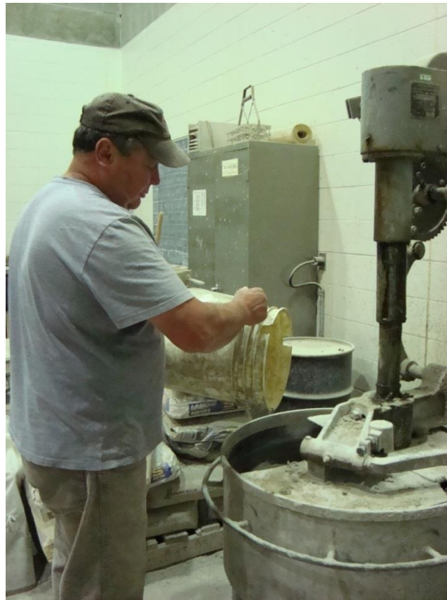
Figure 3.9. Mixer used for mortar preparation
