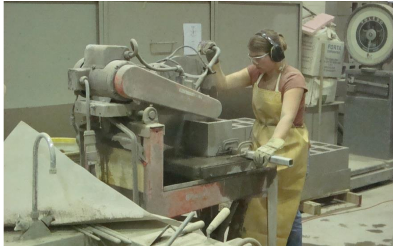
Figure 3.8. Masonry table saw used to cut half blocks
