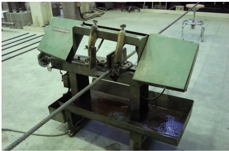
Figure 3.7. Cutting of reinforcing bars with band saw
