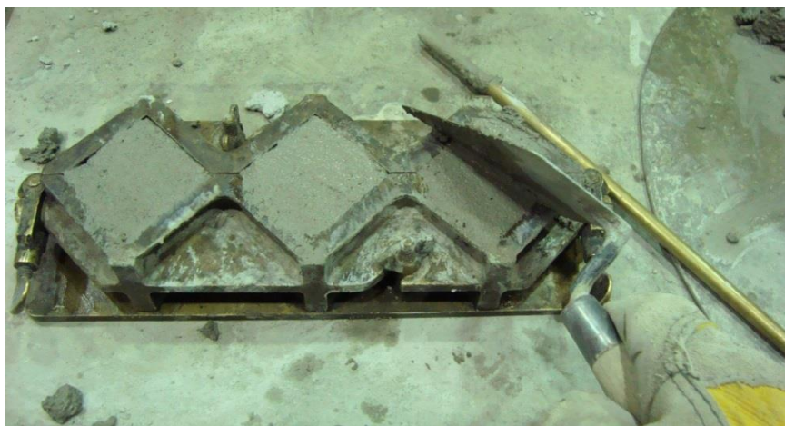
Figure 3.10. Mortar cube preparation
