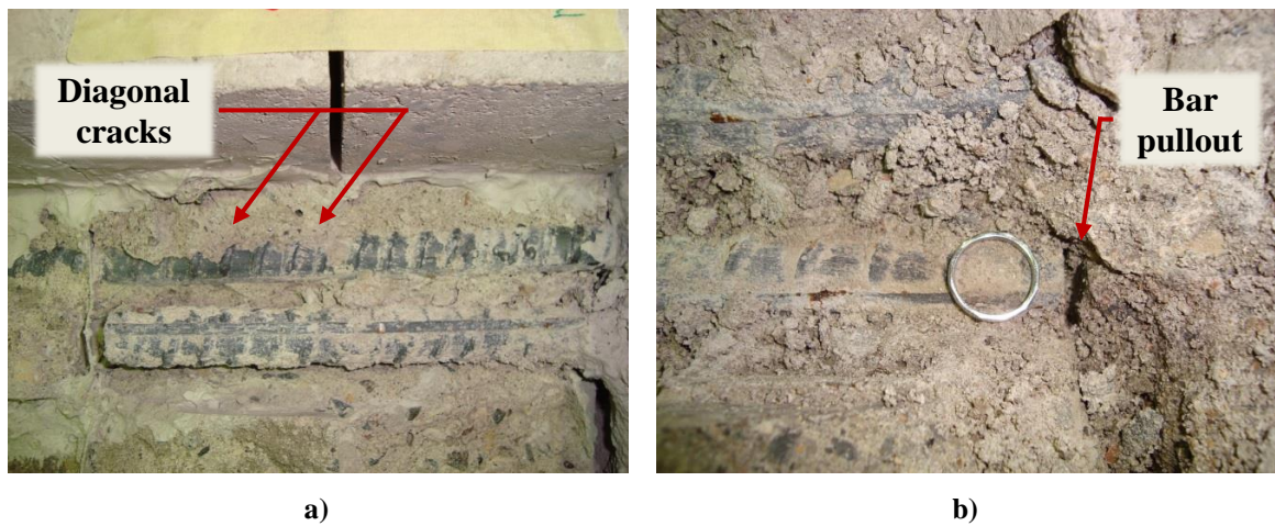
Figure 4.11. Evidence of bond failures in wall splice specimens: a) diagonal cracking in grout surrounding splice reinforcement, and b) bar pullout in lap splice
