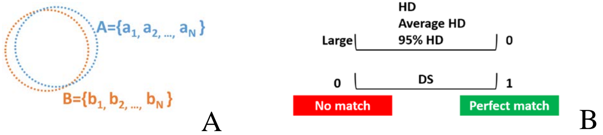
Figure 4. 8 (A) Two datasets, A and B, that help to define HD, average HD, 95% HD, and DS from Equations (4.1) to (4.4); and (B) the evaluation of HD, average HD, 95% HD, and DS in match performance.
