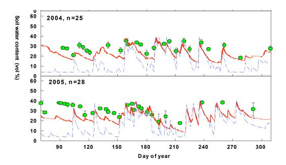
Figure 1. Soil water contents simulated at 0 -5 cm by DSSAT -CSM and at 0 -6 cm by SHAW using hourly weather data and observed at 0 -6 cm using Theta probe in the conventionally tilled continuous wheat in the growing seasons of 2001-2005 at Three Hills, AB.
