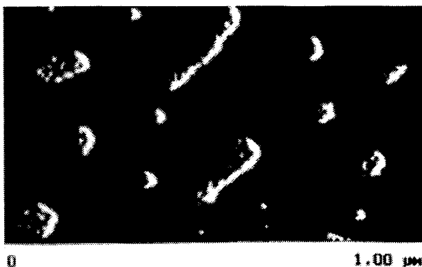
Fig. 1: SFM image of spin-coated humic acid. Height of the deposits: 1.5 to 2 nm.
