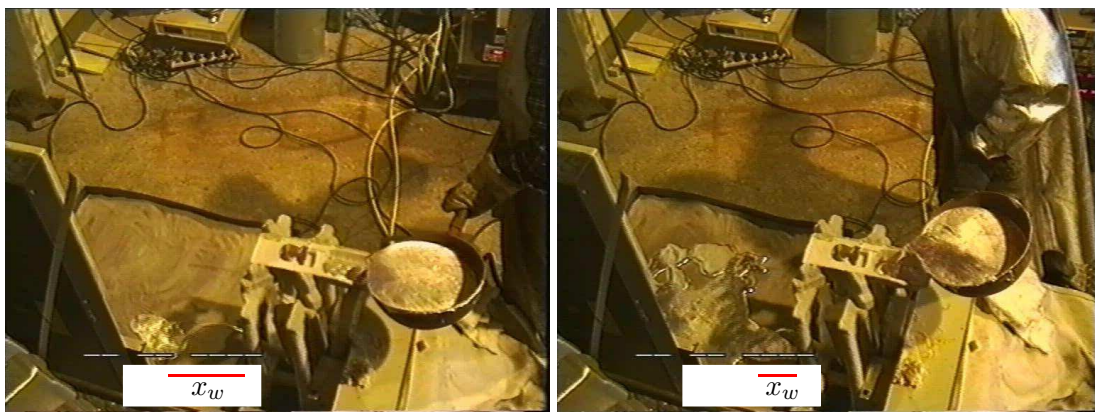
Fig. 6: Braking effect of the magnetic field (shorter outflow parabola)
