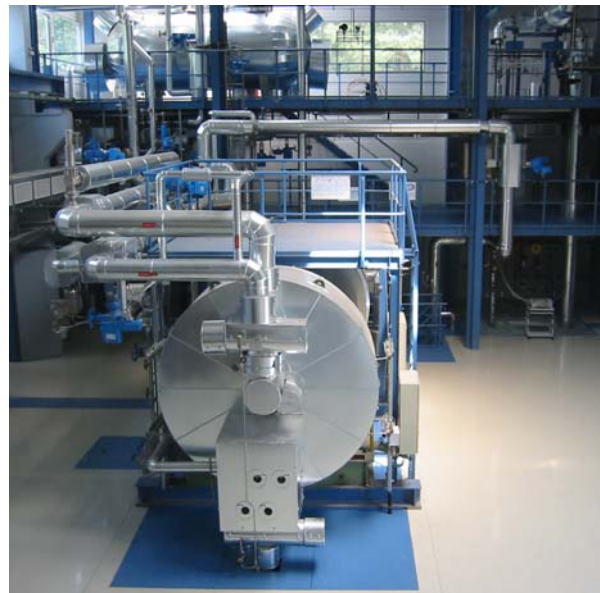
Fig. 4: View of TOPFLOW with the BWR emergency condenser test in the foreground
