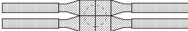
Fig. 1: Mechanical setup of the photon beam monitor. Each scintillator bar is read out by a separate photomultiplier tube via an attached lightguide. The projected photon beam distribution is indicated by a circle.
