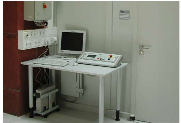
Fig. 2: Control unit of the Isovolt X-ray tube in front of the laboratory.
