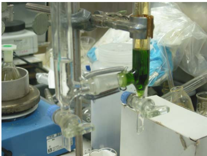
Fig. 3.4.1: Image of the electrolysis cell in the glove box. Cathode-chamber: Pu raw-solution, Anode-chamber: 2 M \text{HClO}_4 .
