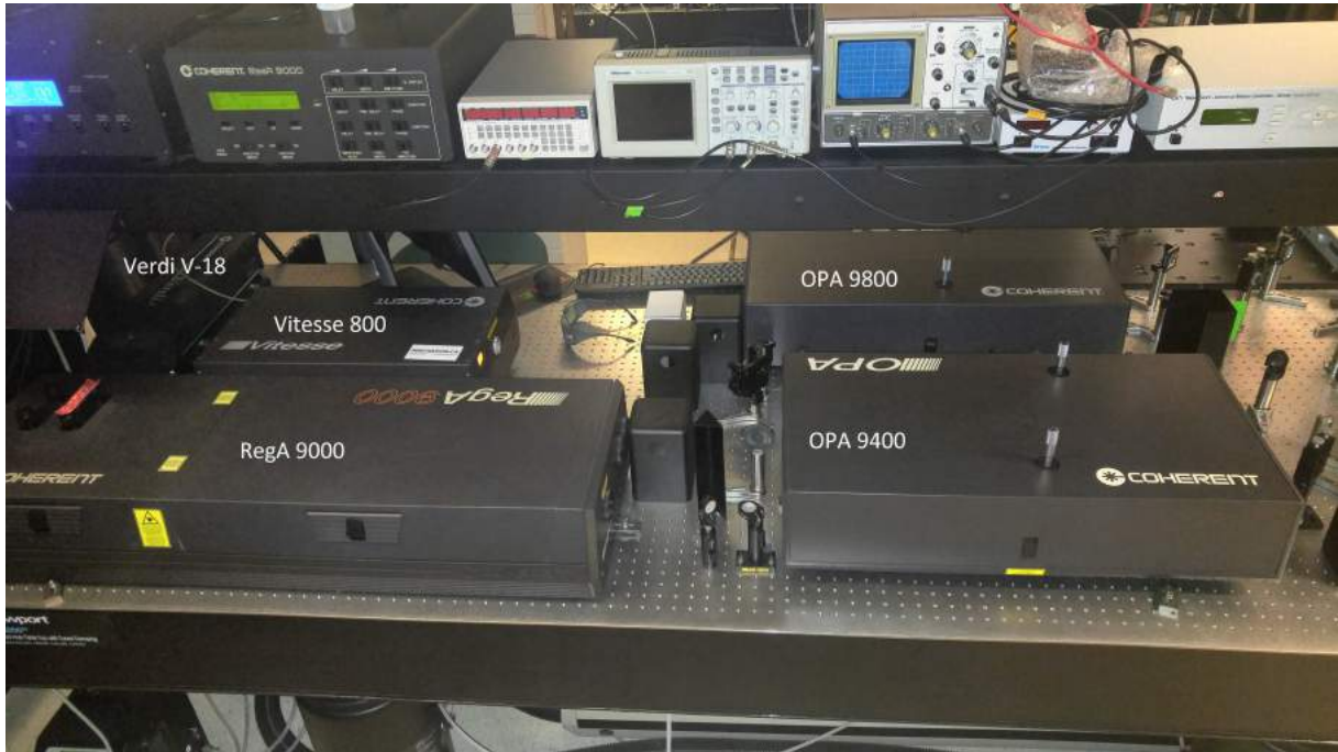
Figure 4.1: Photo of the SSSC SEE laser facility at the University of Saskatchewan. The Verdi, Vitesse, RegA, and OPA units are shown and labelled.
