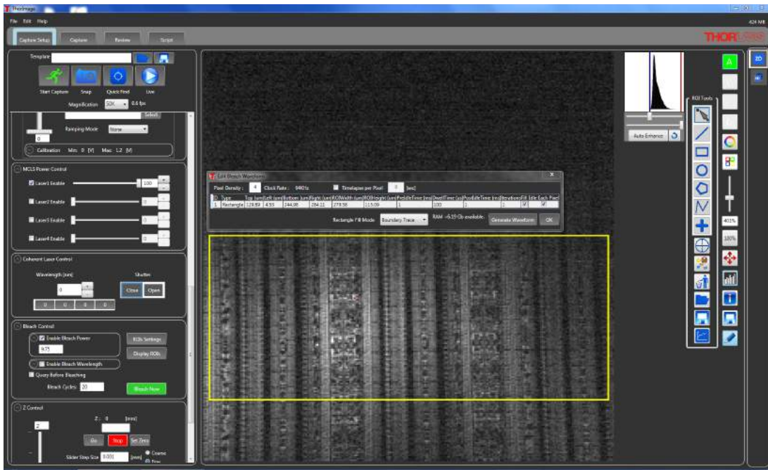
Figure 4.4: Screen capture of the ThorImageLS software version 2.3 with a section of the Virtex-5 configuration memory being imaged by the imaging laser. The yellow box is the rectangular ROI selected.
