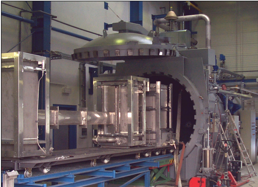
Fig. 5.3: The pressure chamber and the test-section components
