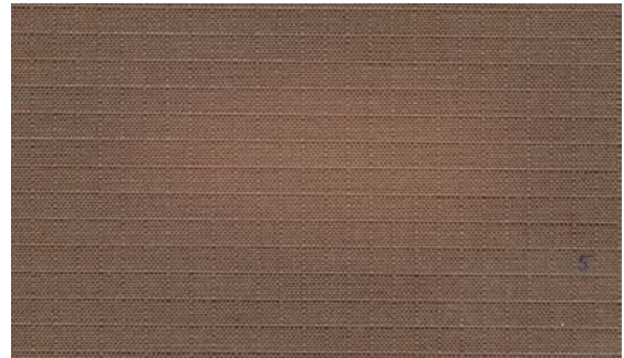
Figure A.2: 1200 s at 5 kW/m 2
