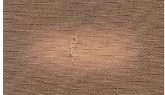
Figure A.8: 240 s at 10 kW/m 2
