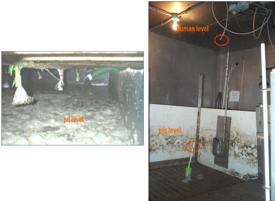
Figure 4.7. Air sampling points in each chamber: pit, animal and human levels.
