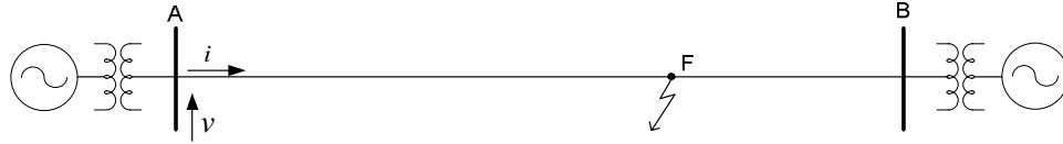
Figure 2.5: Voltage and current at fault inception
