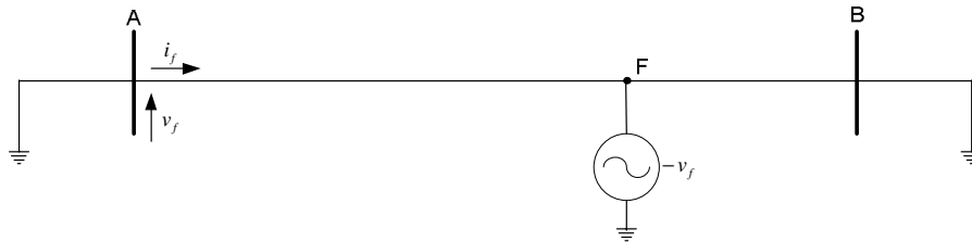
Figure 2.7: Voltage and current components injected by the fictitious source at the fault
