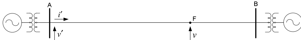
Figure 2.6: Voltage and current before fault
