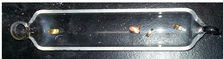
Figure 3.7. Cu foil clippings in a quartz tube ready to enter the furnace tube. The sizes of the clippings were approximately 0.25 cm x 0.25 cm x 0.1 mm.
