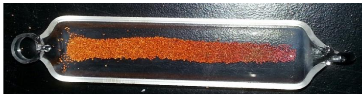
Figure 3.8. Copper pellets (<1 mm) in a quartz tube before heating. The discoloration is due to the lighting and the camera. The copper pellets (< 1mm) are the bright orange color as depicted in the far left of the image.
