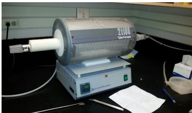
Figure 3.2. The tube furnace used in the thermal oxidation preparations. The end cap through which the air exits is not shown.
