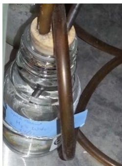
Figure 3.1. Preparation of a H 2 S through bubbling.
