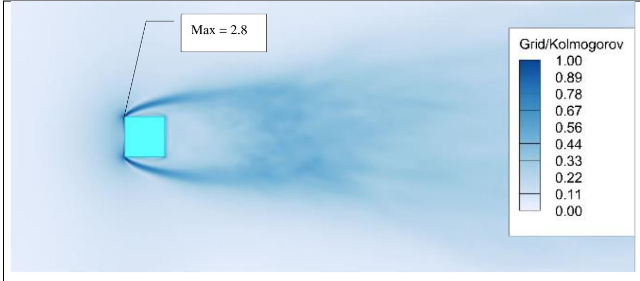
Figure 3.4. Ratio of grid size to Kolmogorov length scale in the horizontal ( X - Z ) mid-plane predicted by the DNM.
