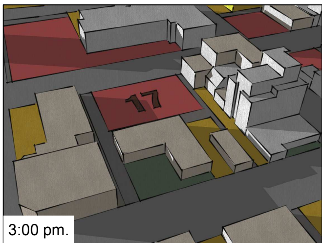
Figure 34: Shadow simulation for lot #17 shows numerous places within the lot and nearby alleys where solar exposure is preserved.
