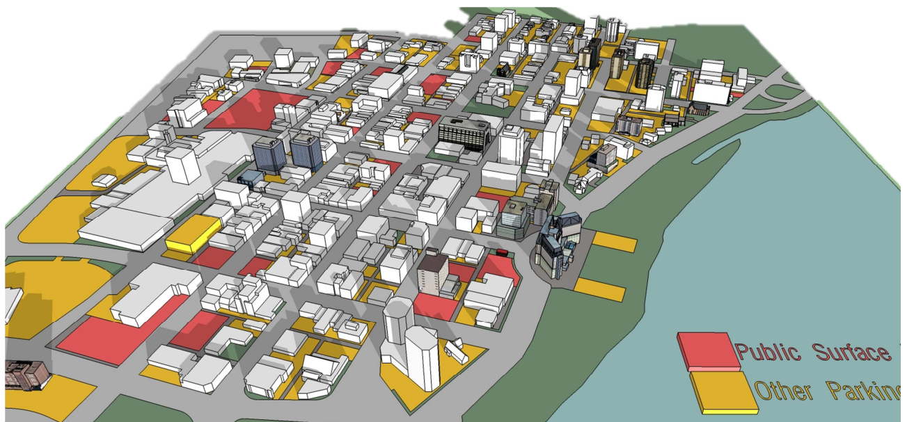
Figure 16: Google® SketchUp model of Saskatoon's CBD. This model was created to estimate shadow patterns in back alleys and other spaces throughout downtown.
