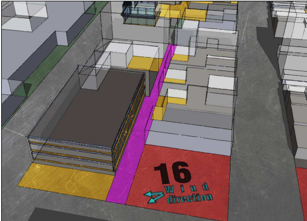
Figure 25. Lot #16 is oriented almost perpendicular to the prevailing wind; as well the building heights along the back alley are fairly evenly distributed, lessening the potential for downward gusts of wind.
