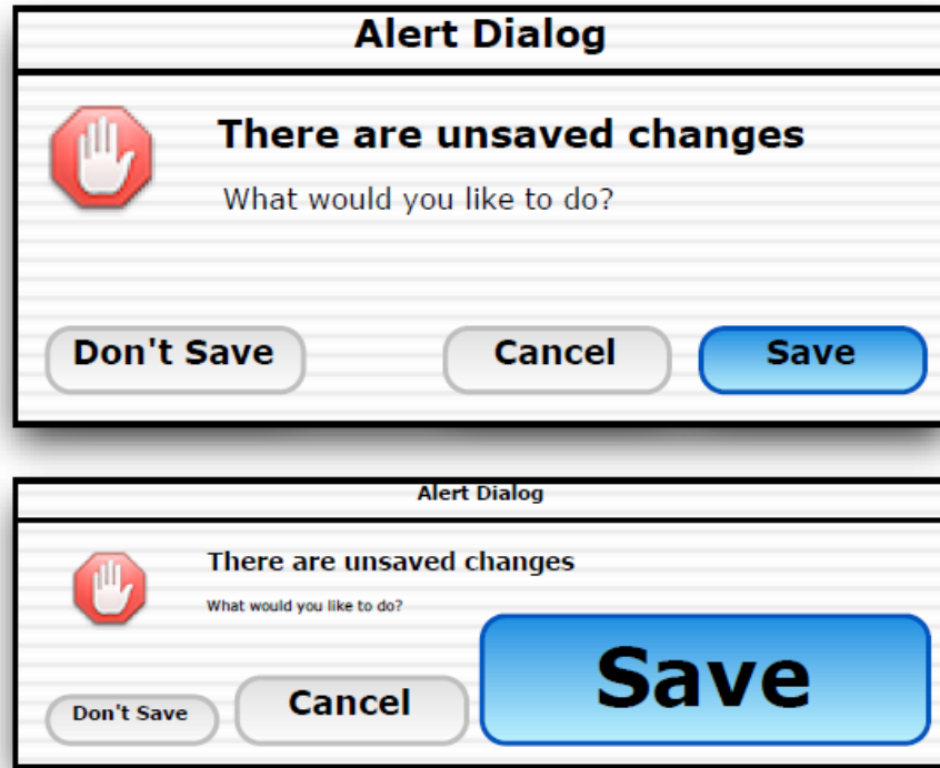
Figure 2.4: An example of Sticky Targets. The top image is the visual representation of the dialog, the bottom image is the dialog representation in motor space
