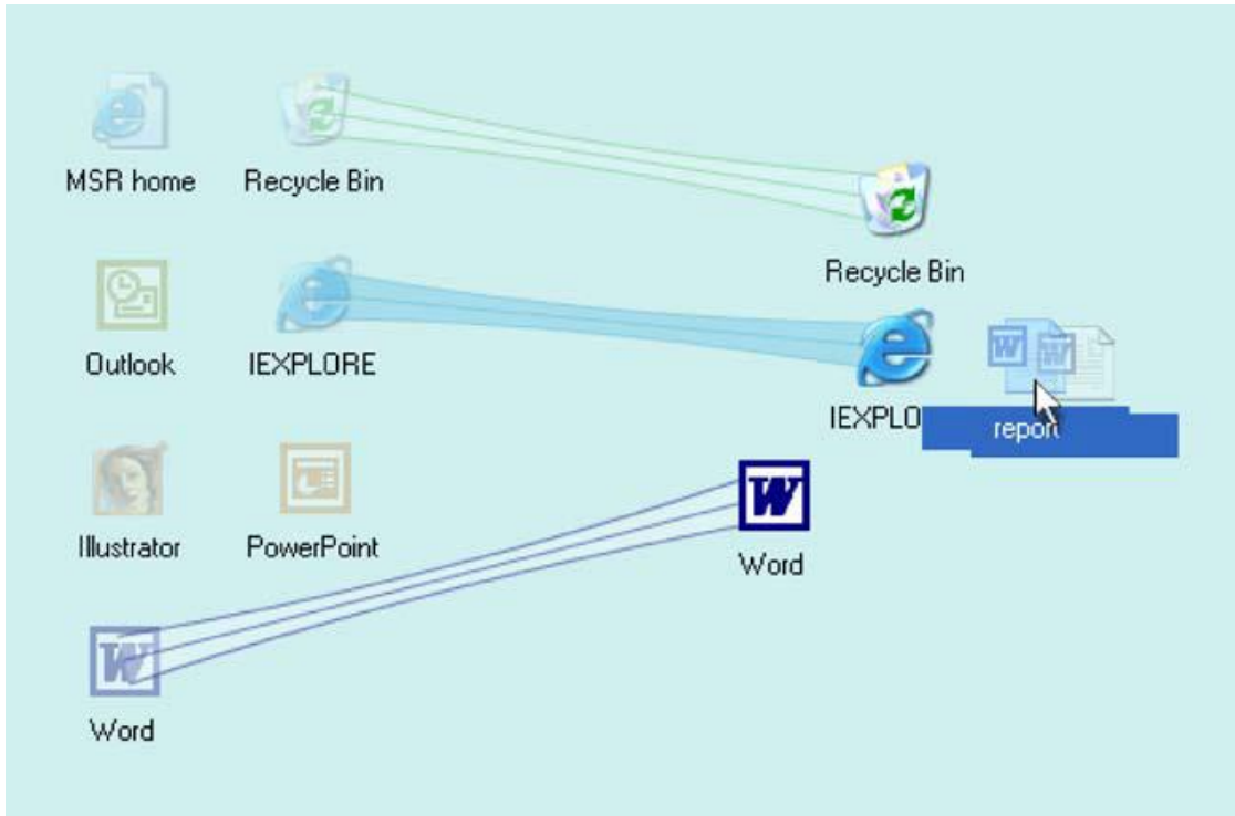
Figure 2.3: Drag and pop technique – “virtual proxies” of the icons are brought closer to the cursor
