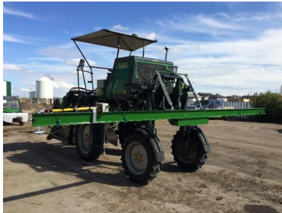
Figure 2.7: 1 st Generation Boom Assembled with Sensors
