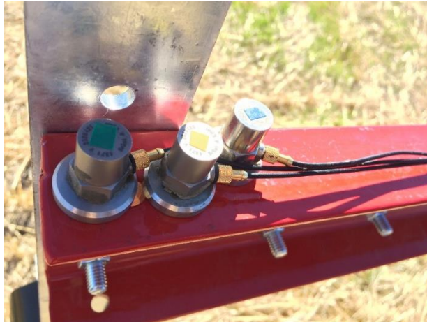
Figure 3.22: Sensor Location of Natural Frequency Measurements Performed on 2 nd Gen Boom
