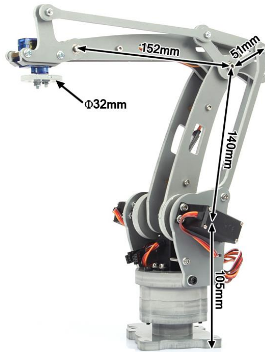
Figure 4.16: Robotic Arm for Verifying the Kinematics
