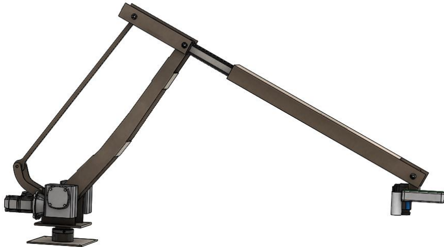
Figure 4.8: Schematic of the Proposed 3 rd Generation Boom for Plant Phenotyping.
