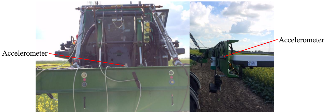
Figure 3.7: Sensor Located at the Center (Vertically) and Left End (Horizontally) of the Boom
