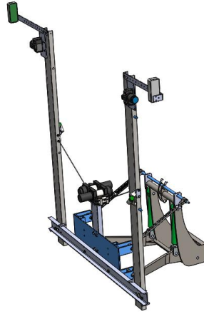
Figure 2.14: Assembly of Developed 2 nd Generation Boom in Folded Configuration
