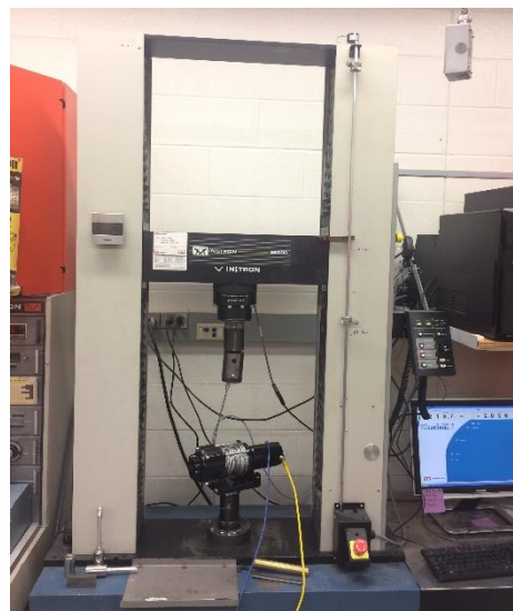
Figure 2.22: Universal Testing Machine for Pulling Capacity Tests
