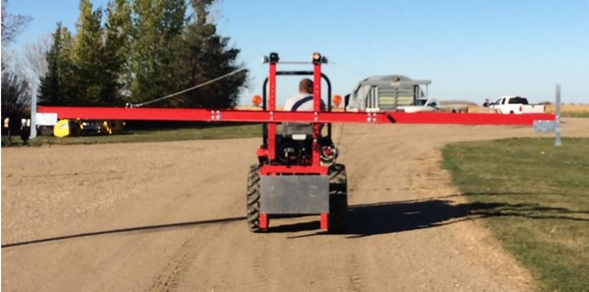
Figure 3.29: 2 nd Generation Boom Mounted on a 4ft-Tractor in the Vibration Test
