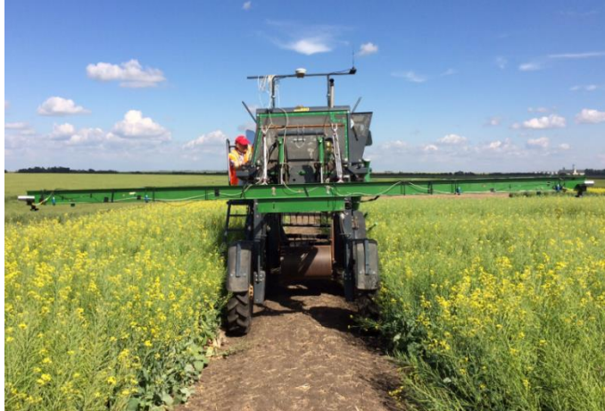
Figure 3.6: Overall Setup for 1 st Generation Boom Field Vibration Experiments
