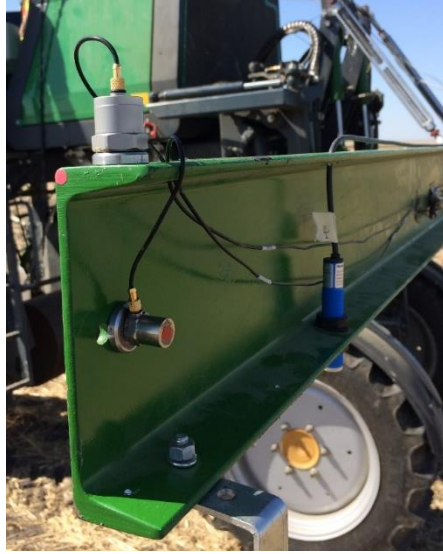
Figure 3.15: Vertically and Horizontally Mounted Sensors at the Left End of the 1 st Gen Boom
