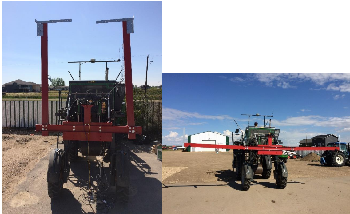
Figure 2.23: 2 nd Generation Boom Mounted on a Swather (Type A in folded, and expanded boom positions)
