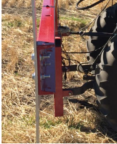
Figure 2.13: 3-Point Hitch Connection between 2 nd Generation Boom (Type B) and Tractor
