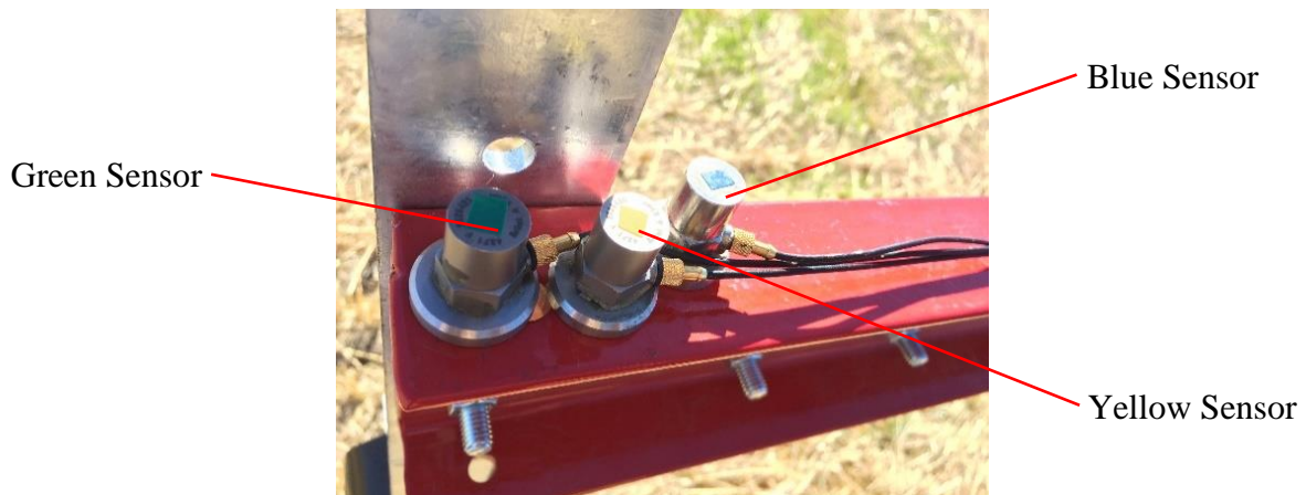
Figure 3.10: Sensors Located at Left End of the Boom Vertically
