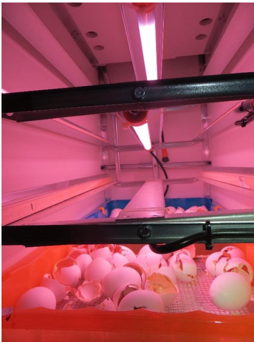
Figure 4.1. LED lights outfitted into a 1502 Sportsman incubator.
