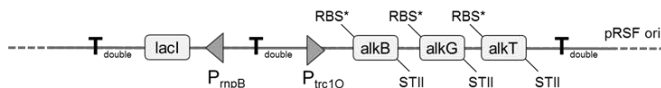
Figure 3.2: Schematic representation of the constructed expression system of the plasmid pAH042. RBS* = ribosomal binding site optimized for Synechocystis sp. PCC 6803 (Heidorn et al. , 2011), STII = Strep-tag II (Schmidt et al. , 1996), T double = double terminator (biobrick #BBa_B0015).
