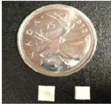
Fig. 4.18 1.29mm thick polymer ceramic DRA samples (DRA samples courtesy of M. Tayfeh)
