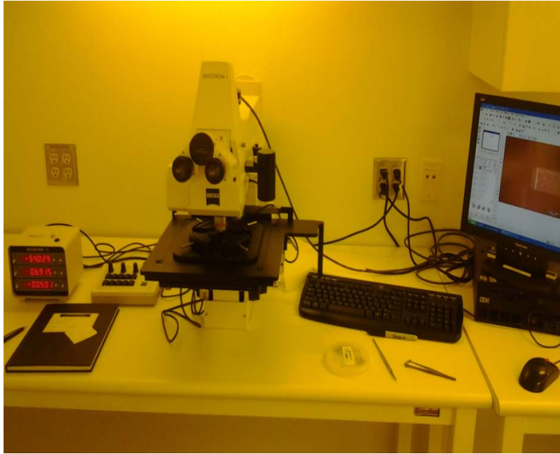
Fig. 3.15 Measurement platform: Zeiss Axiotron 1 Microscope
