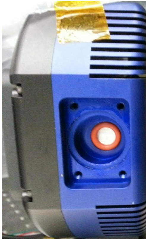
Figure 5-1: The QSI CCD with the panel that covers the vacuum seal removed. The orange o-ring seen in the cavity is removed from the chamber to break the vacuum seal on detector.
