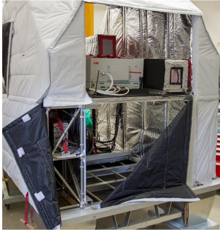
Figure 5-2: The ALI instrument is mounted on board the CARMEN-2 gondola (top shelf on the right). ALI located next to SHOW. ALI has a cover over the optical entrance to protect the instrument from dust and other contaminants. Thermal insulation has been added to the instrument exterior. Some of the reflective covering was blacked out to not cause additional stray light into SHOW optical path.
