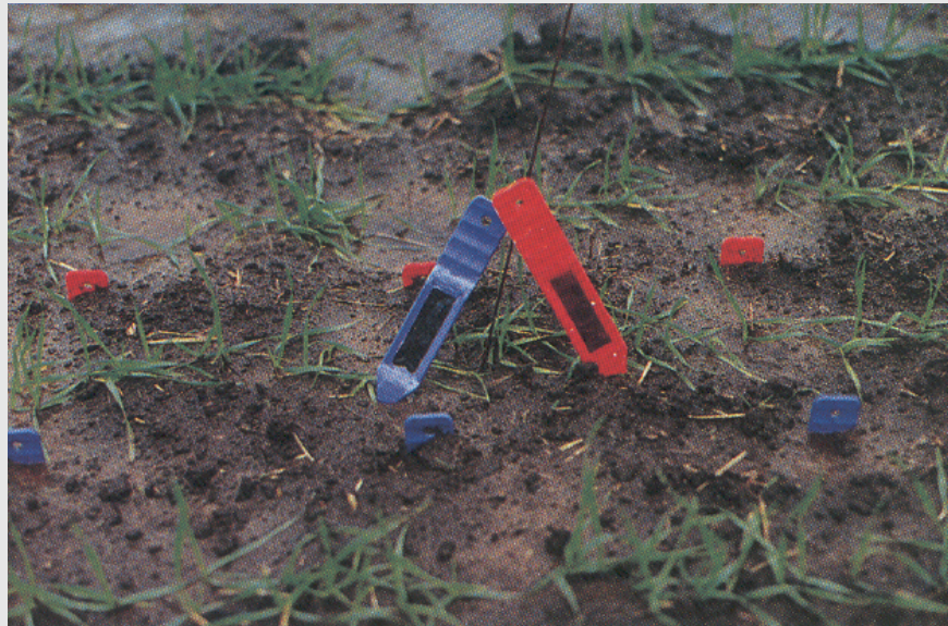
Figure 1. PRS™ Probes inserted directly into a moist field soil.
