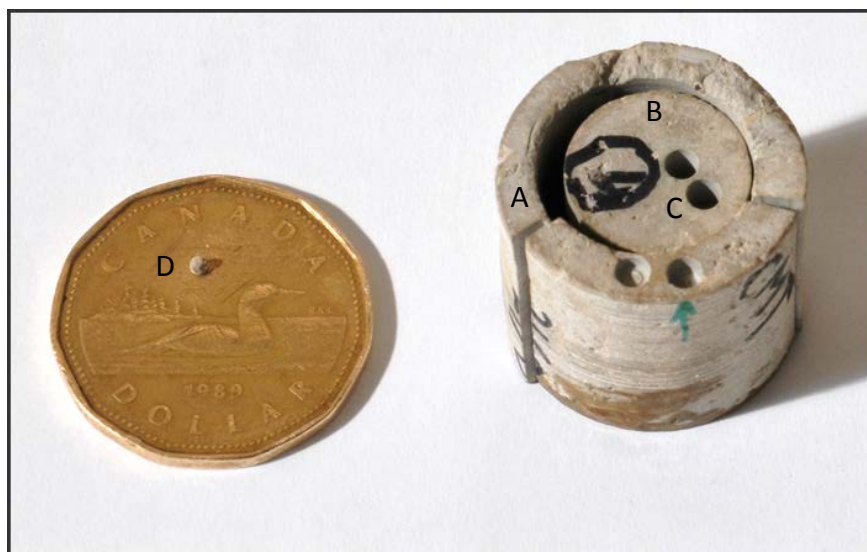
Figure 1.5 Sample cores with similar dimensions to KD-18-03. (A) Large diameter core used in petrophysical laboratory measurements. (B) Core used in 10 \mu\text{m} CMT analysis. (C) Hole that was drilled to obtain the sample D. (D) Representative region of the core region used for 0.78 \mu\text{m} CMT based core analysis. The reference object is a Canadian dollar which has a diameter of 26.5 mm (Royal Canadian Mint, 2012).
