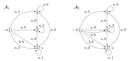
Note that  $A_2$  was constructed by inserting a transition (1, b, 3) into  $A_1$ .
