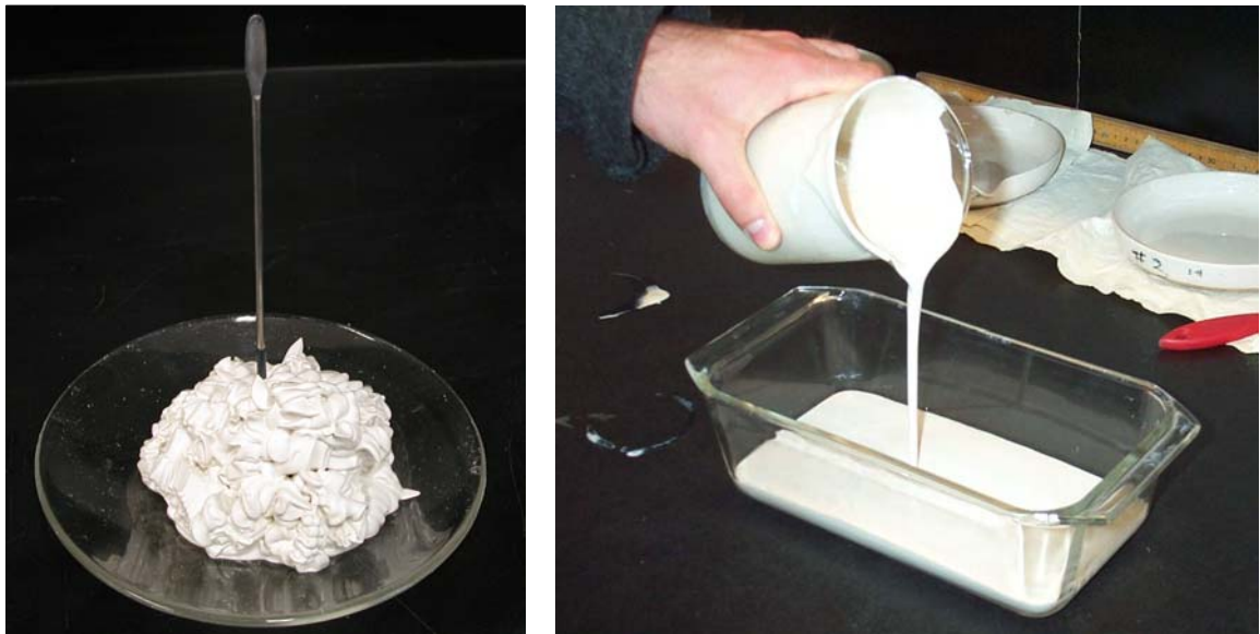
Figure 4.15: Effect of adding TSPP to Dry Branch Pioneer kaolin clay slurry 19% by volume with a measured Bingham yield stress of 128 Pa.
