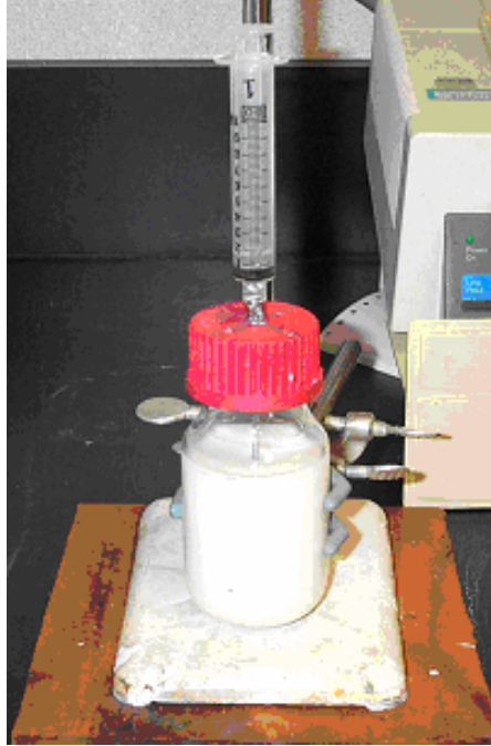
Figure 3.3. Picture of Modified Andreasen Sedimentation Pipette used in centrifuge sedimentation.
