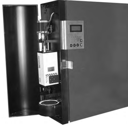
Figure 3.6: A prototype of readout set-up for two-dimensional thermally stimulated dosimetry. After [32].
