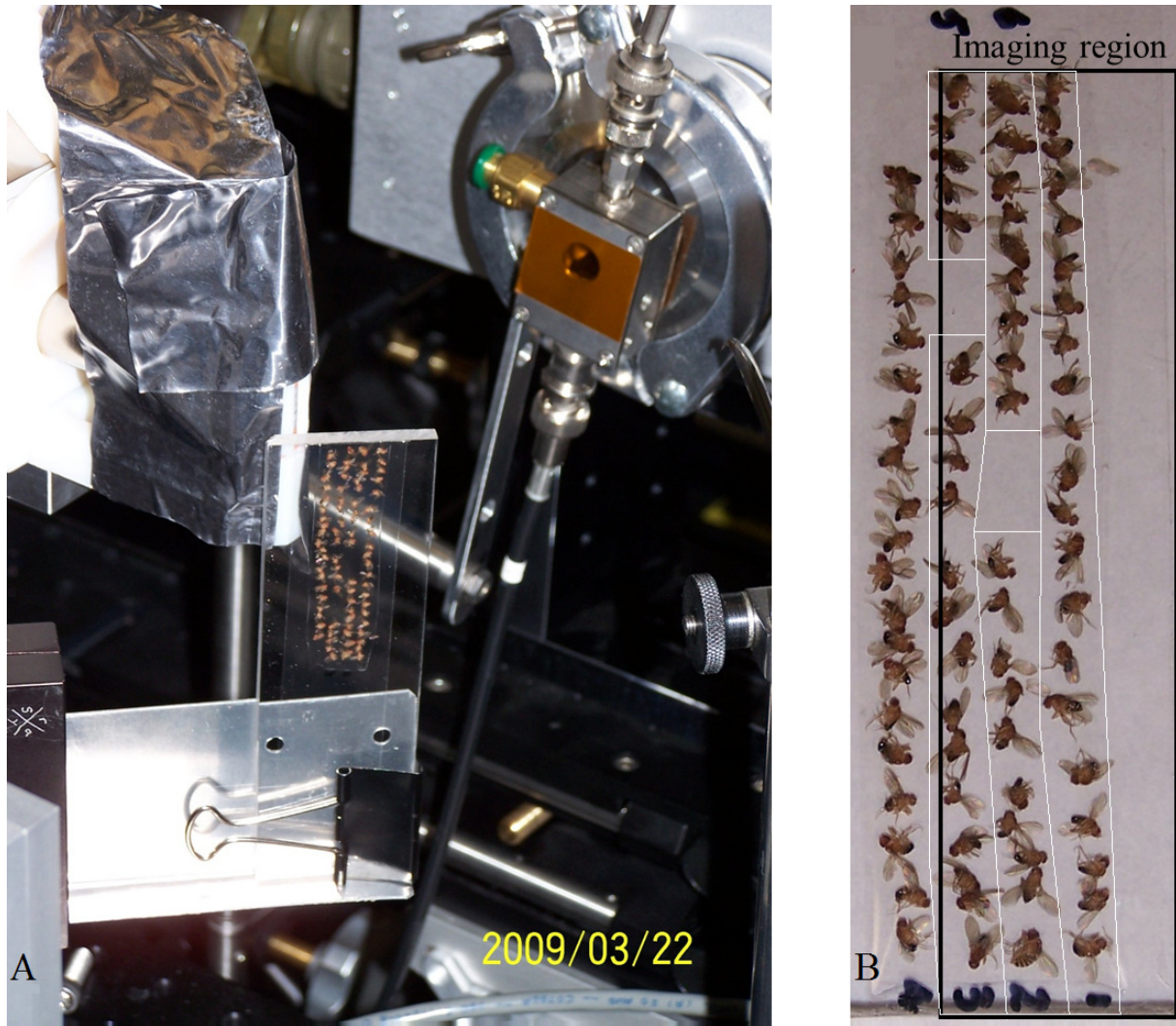
Figure 4.25 Drosophila sample in the imaging setup (A) and the Drosophila sample photo (B) noted with the imaging region (black rectangle) and the Drosophila packing groups (while lines) with group numbers (1 - 6).
