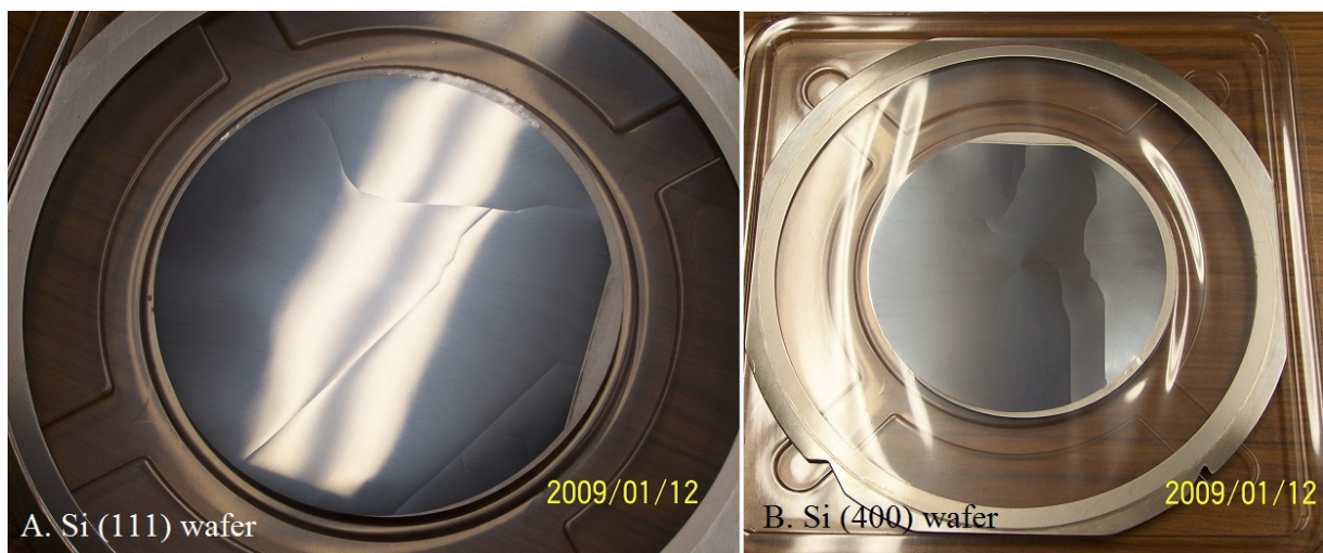
Figure 4.11 Si wafers out of box with 150 mm diameter and 20 \mu\text{m} thickness.
