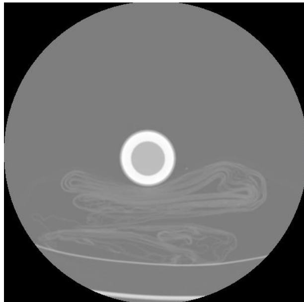
Figure 3.7 An image of a phantom scanned at the same time with the first rat for CT image calibration. The phantom is made of a plastic tube of distilled water placed in another plastic tube of calcium chloride ( \text{CaCl}_2 ) solution.
