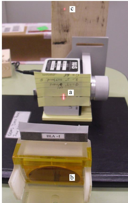
Figure 4.44 Checking the BLA bending through measurement of the reflection focus (c) from the crystal surface (b) using a line laser source (a).
