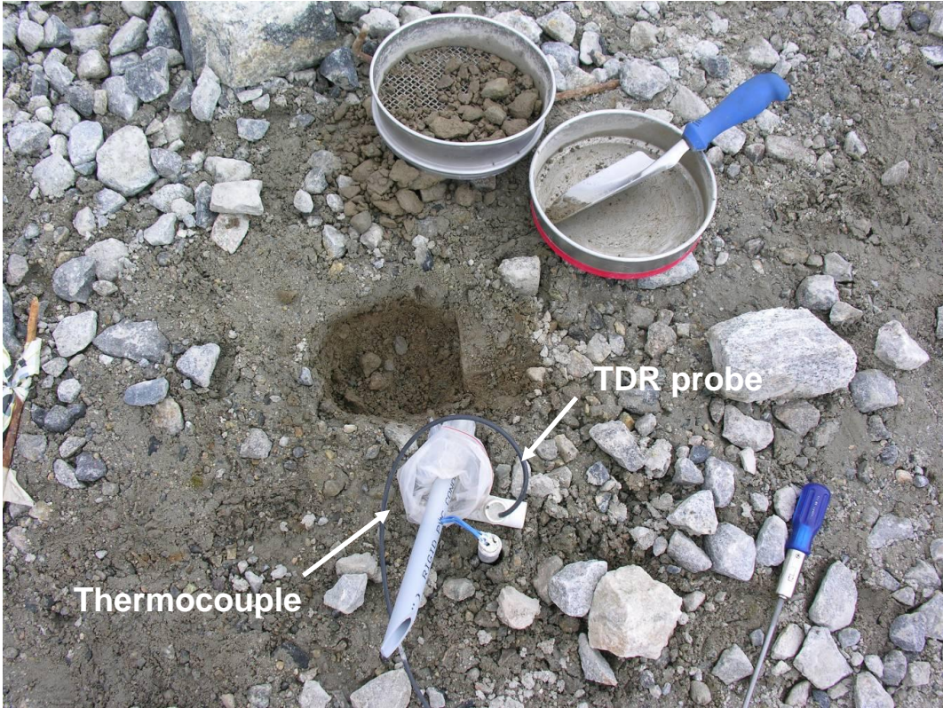
Figure 3.2 Thermocouple and time domain reflectometry (TDR) probes were installed at each sampling location to collect soil temperature and liquid water content at each sampling time.
