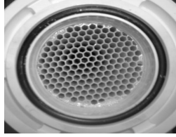
Figure 2.13: A honeycomb flow conditioner located upstream of the orifice plate in the RAMEE test facility
