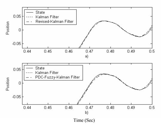
Figure 6.9 Expanded View for Comparing Position Estimations (cm)
