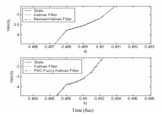
Figure 6.10 Expanded View for Comparing Velocity Estimations (cm/s)
