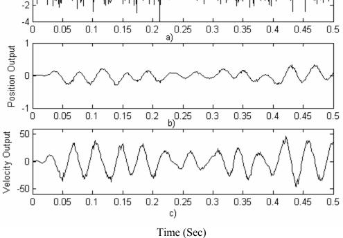
Figure 6.13 Input and Outputs beyond the Assumed Measurement Noise Covariance
