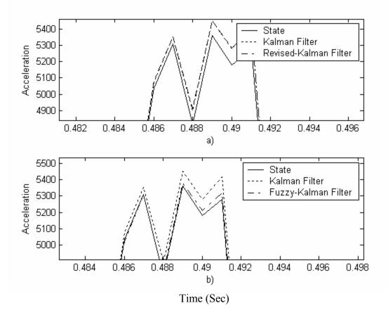
Figure 6.16 Expanded View for Comparing Acceleration Estimations (cm/s<sup>2</sup>)
