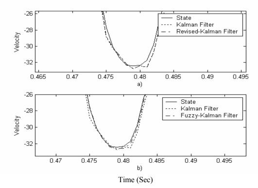
Figure 6.15 Expanded View for Comparing Velocity Estimations (cm/s)
