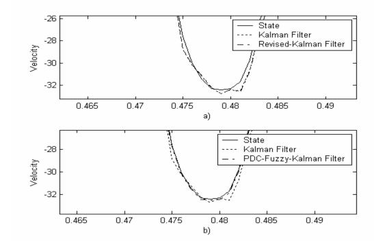
Time (Sec) Figure 6.19 Expanded View for Comparing Velocity Estimations (cm/s)
