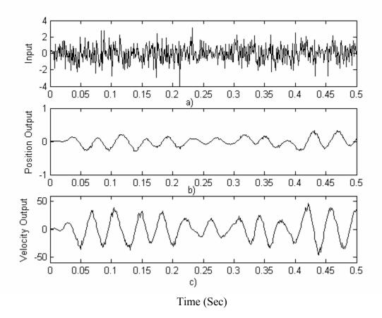
Figure 6.17 Input and Outputs beyond the Assumed Measurement Noise Covariance
