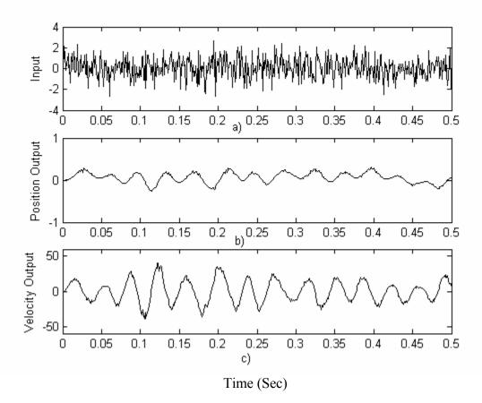
Figure 6.22 Input and Output Signals beyond the Assumed Noise Covariance
