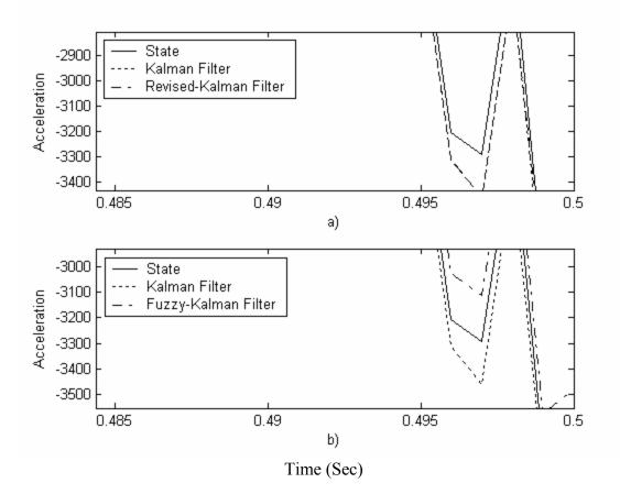
Figure 6.28 Expanded View for Comparing Acceleration Estimations (cm/s<sup>2</sup>)
