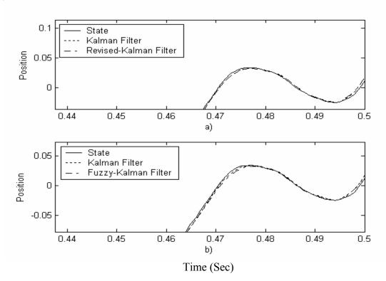
Figure 6.5 Expanded View for Comparing Position Estimations (cm)
