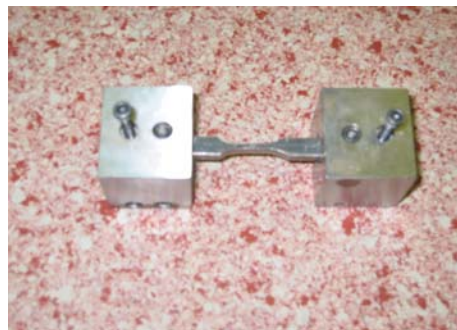
Fig.4. Type L tensile-impact specimens.
