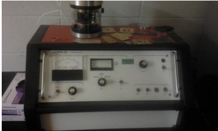
Figure 3.3 Hummer VI sputtering system
