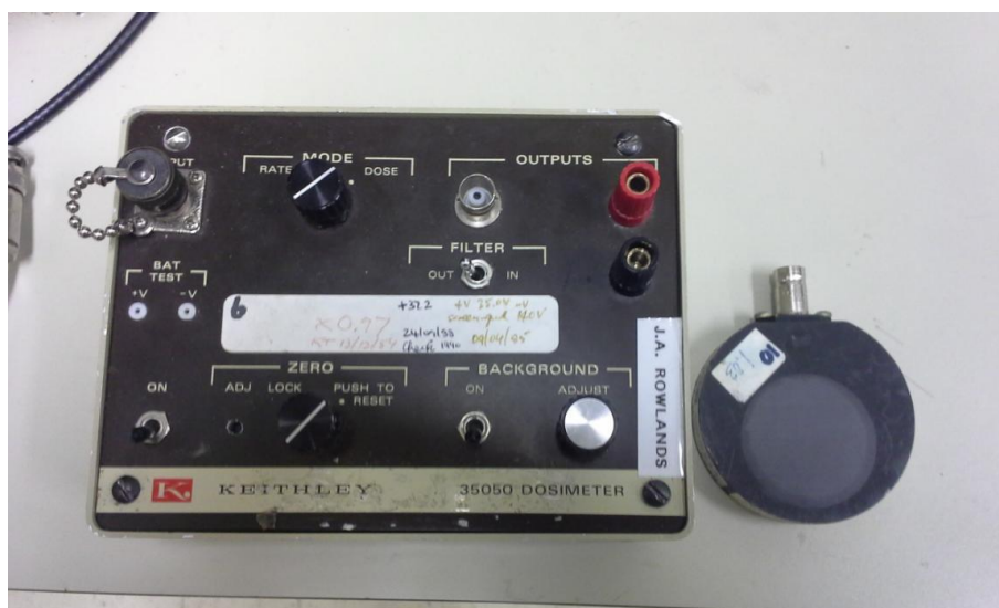
Figure 3.6 Keithley 35050 Dosimeter and Ion Chamber for X-ray exposure measurement
