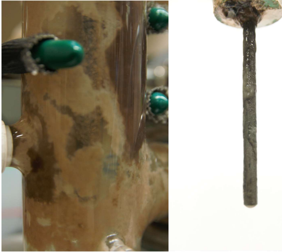
Figure 3.19 Biomass attached to the surfaces of the anodic chamber wall and single rod electrode as result of lactate biodegradation in the MFC fed continuously with 5,000 \text{ mg L}^{-1} lactate with loading rates up to 4800 \text{ mg L}^{-1} \text{ h}^{-1} .
