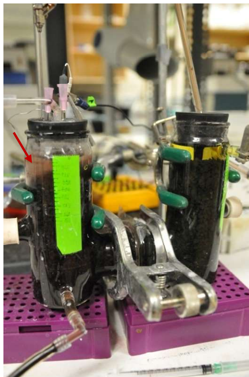
Figure 5.3 MFC with granular graphite electrode with added neutral red as mediator operated batchwise. Arrow indicates red stain around the chamber.
