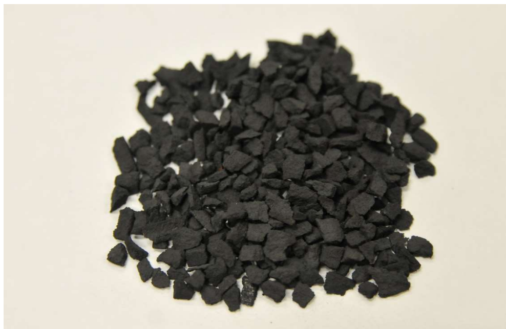
Figure 4.1 Graphite granules used as electrode in MFC.
