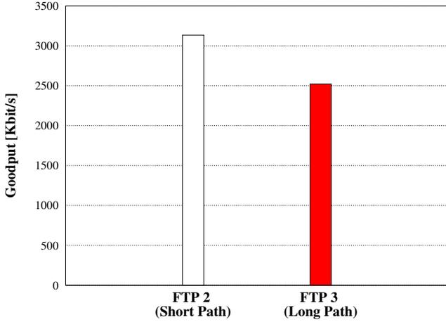
**Figure 3:** Goodput of FTP 2 and FTP 3 without background traffic of FTP 1
