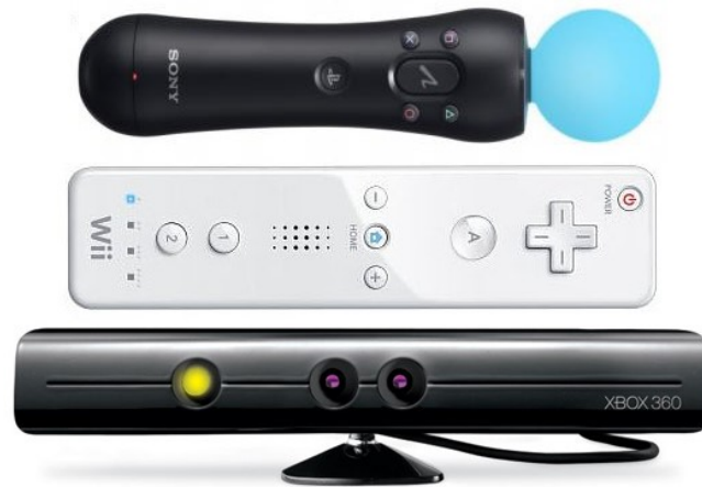
Figure 2.20: New video game input devices. Playstation Move on top, Nintendo Wiimote in middle, and Microsoft Kinect on bottom [88].
