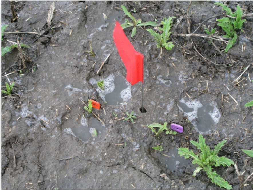
Figure 3. Plant Root Simulator-probes™ used to measure the effects of broadcasted liquid hog manure on soil nutrient availability. (Photo courtesy of Dr. Ken Van Rees)
