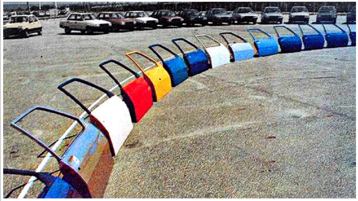
Figure 5-9 In the former time, colors are applied on parts for assessment [Lee, 2007]
