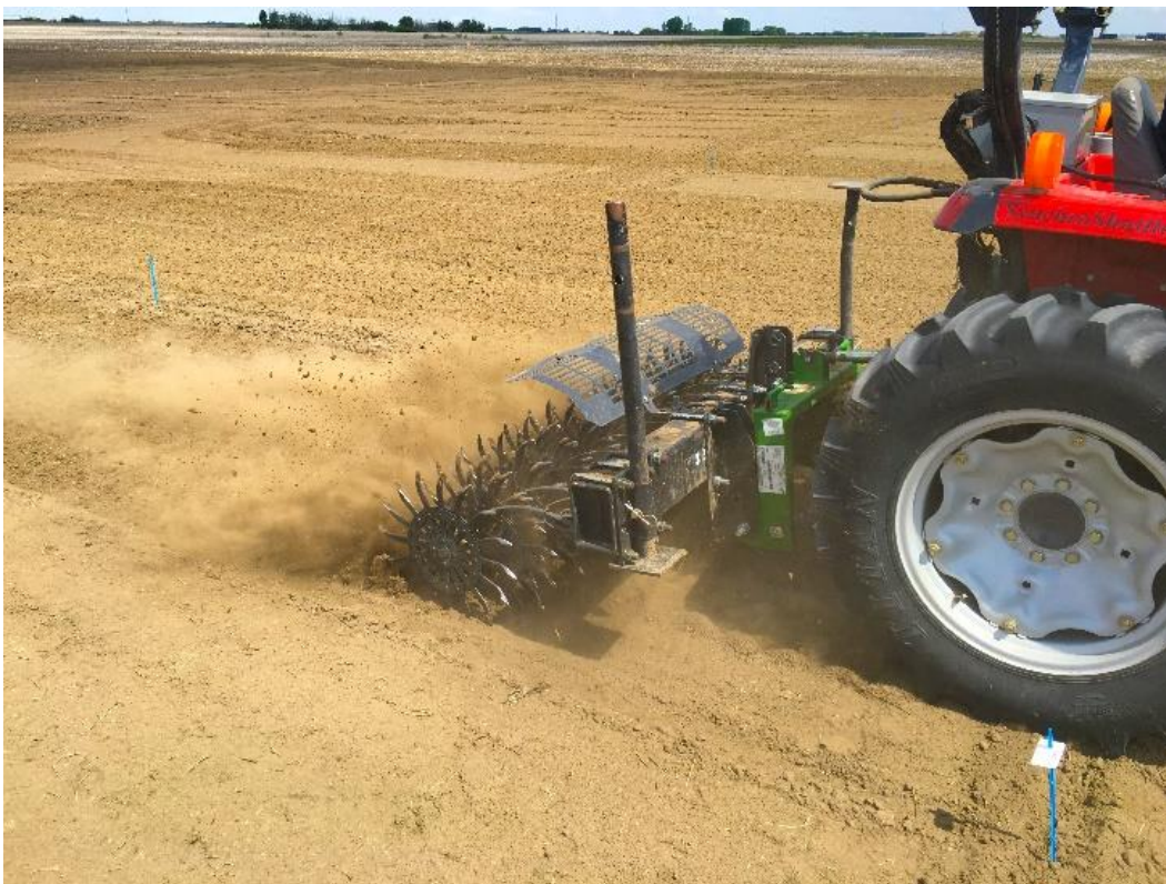
Figure 2.1 A minimum-tillage rotary hoe in operation (Photo credit: Oleksandr Alba)
