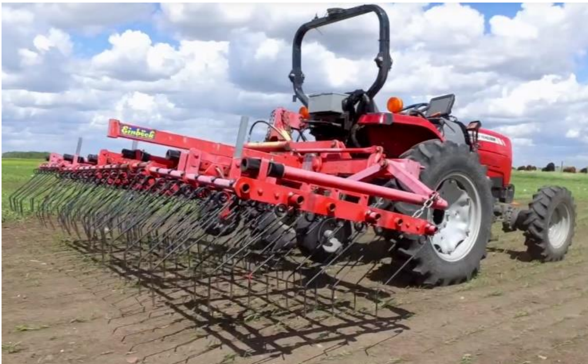
Figure 2.3 The spring tine “Einbock” harrow (Photo credit: Oleksandr Alba)
