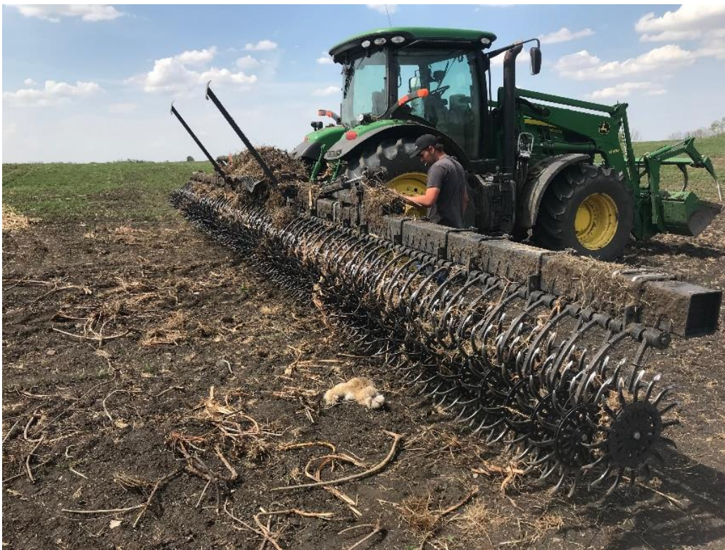
Figure 2.2 Cleaning of the minimum tillage rotary hoe after operation in high residue fields. (Photo credit: Oleksandr Alba)
