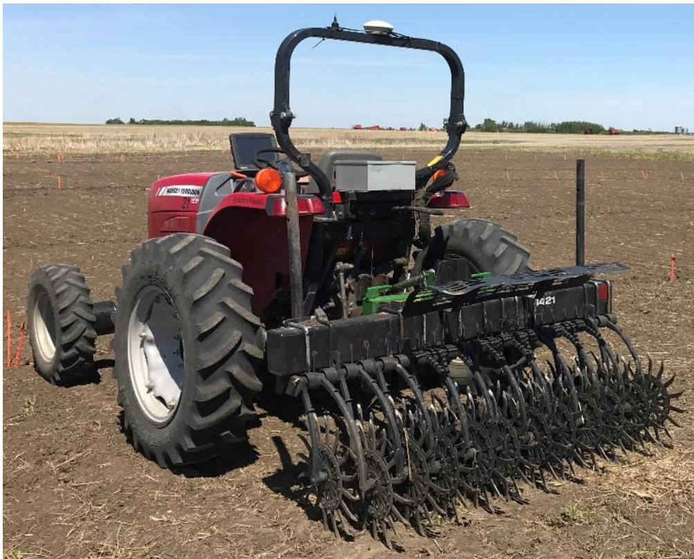
Figure 3.1 The minimum-tillage (min-till) “Yetter” rotary hoe.
