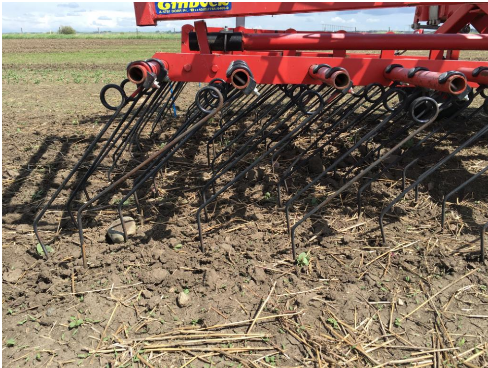
Figure 3.2 The flex-tine harrow tine angle adjustment.
