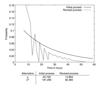
Figure 7. Probability distributions and statistical measures of the alternative processes
