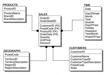
Fig. 4. Star schema of data warehouse dw1
