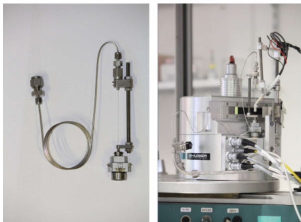
Figure 3.3: Laboratory in situ X-ray powder diffraction; Sample mounting and gas attachment (left) and set up at the Giunier camera (right). Heating is realised by a resistivity heater.
