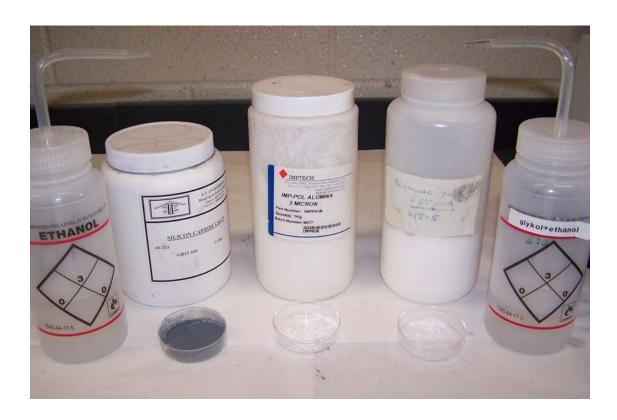
Figure 4.5: Some of the materials used for polishing. Left to Right: 100% Ehanol, Silicon Carbide powder, 3 micron alumina powder, 0.05 micron alumina powder and Ethanol+Glykol mixture.
