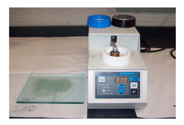
Figure 4.3: Left: Glass plate used for grinding. Right: MINIMET 1000 – Polisher.
