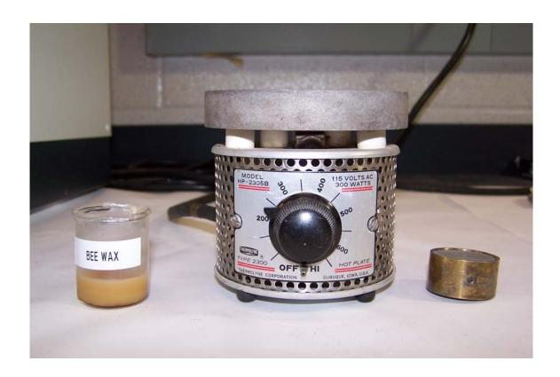
Figure 4.4: Left to Right: Bee Wax, Thermolyne, HP 2305 B Heater, Sample Holder.
