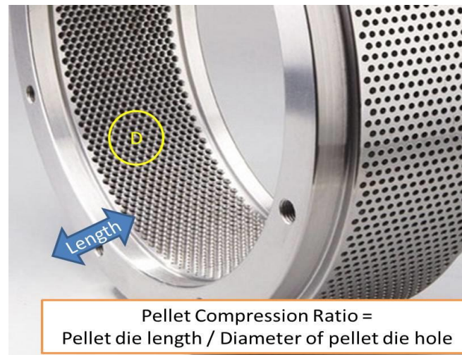
Figure 2.1 Illustration of pellet compression ratio (Chao, 2010)
