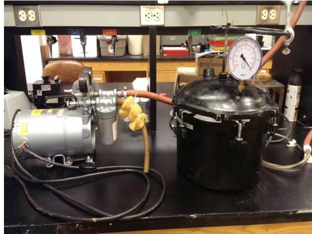
Figure 3.1 Experimental vacuum coating system
