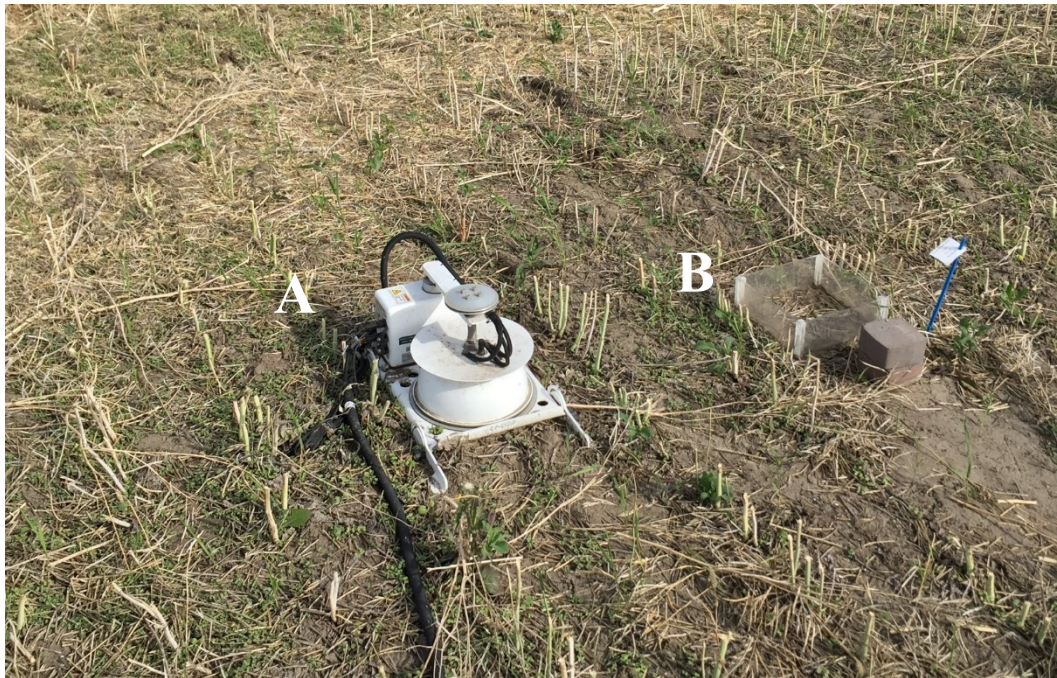
Figure 3.1. Photo showing (A) the AFC-FTIR automated gas sampling chamber and (B) the MFC-GC manual gas sampling chamber in the field.
